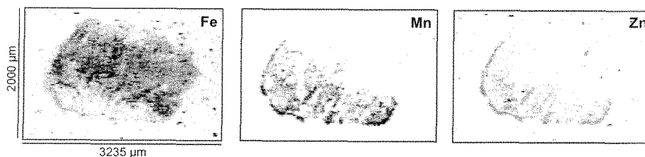
Figure 1. Gray-scale \mu\text{SXRF} maps in negative contrast showing the distribution of Fe, Mn and Zn in the uncontaminated soil. The Fe and Mn maps were collected at 10 keV, and the Zn map was obtained by subtracting the normalized fluorescence signal recorded 50 eV above and below the Zn K-edge to eliminate any noise. Beam size: 16\mu\text{m} \times 5\mu\text{m} ; step sized: 20\mu\text{m} \times 20\mu\text{m} ; dwell time: 400 ms/point.
